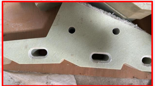
Machining of Insulator for Generator
